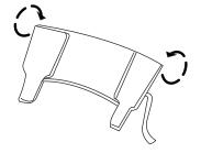
1. Position the boot right-side up and fold each side of the boot inward.
